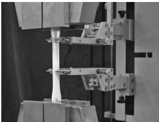
FIGURE 10.10 Extensometer for plastic test coupons.
