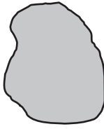
FIGURE 1.33 Torsional constant for a solid section.
