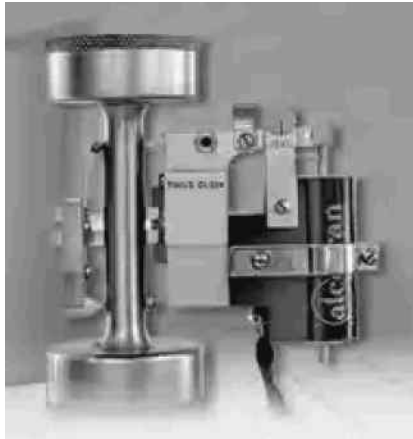
FIGURE 10.11 Extensometer for metal test coupons.
