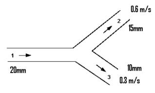
Total mass flow into the junction = Total mass flow out of the junction
